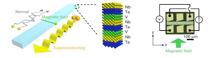
Demonstration of magnetically controllable **superconducting diode**: alternating switching between super- and normal-conducting state by **changing the sign of the applied current or a small magnetic field**
