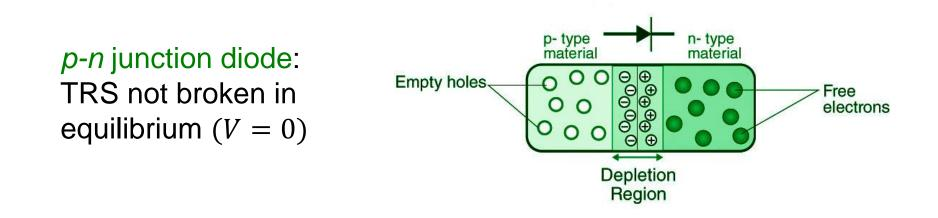
**Rectifiers** are usually based on semiconductor diodes: convert alternating EM field into directed current
